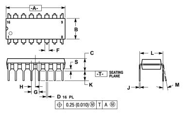
NOTES: 1. DIMENSIONING AND TOLERANCING PER ANSI Y14.5M, 1982. 2. CONTROLLING DIMENSION: INCH. 3. DIMENSION L TO CENTER OF LEADS WHEN FORMED PARALLEL. 4. DIMENSION B DOES NOT INCLUDE MOLD FLASH. 5. ROUNDED CORNERS OPTIONAL
