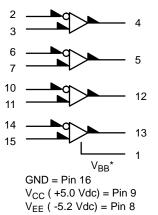
$^*V_{BB}$  to be used to supply bias to the MC10H125 only and bypassed (when used) with 0.01  $\mu F$  to 0.1  $\mu F$  capacitor to ground (0 V).  $V_{BB}$  can source < 1.0 mA.
