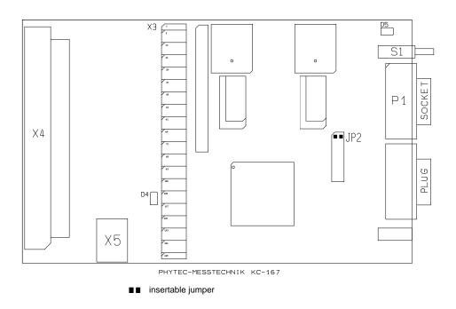
Figure 3: Important jumper and connectors for starting
