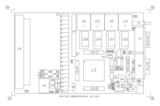
Figure 2a: View of the kitCON-167 (component side)
