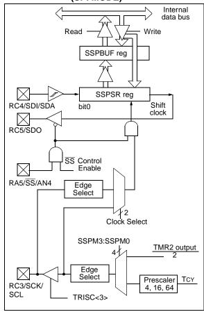
To enable the serial port, SSP enable bit, SSPEN (SSPCON<5>) must be set. To reset or reconfigure SPI mode, clear bit SSPEN, re-initialize the SSPCON register, and then set bit SSPEN. This configures the SDI, SDO, SCK, and  $\overline{\rm SS}$  pins as serial port pins. For the pins to behave as the serial port function, they must have their data direction bits (in the TRISC register) appropriately programmed. That is:
