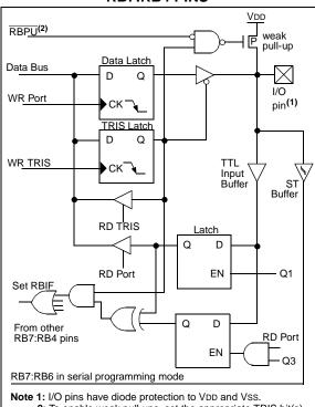
2: To enable weak pull-ups, set the appropriate TRIS bit(s) and clear the RBPU bit (OPTION\_REG<7>).
