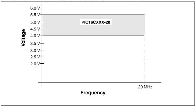
FIGURE 16-2: PIC16LC63A/65B/73B/74B VOLTAGE-FREQUENCY GRAPH
