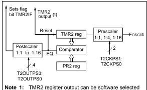
Note 1: TMR2 register output can be software selected by the SSP module as a baud clock.
