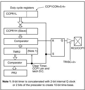
A PWM output (Figure 9-4) has a time base (period) and a time that the output stays high (duty cycle). The frequency of the PWM is the inverse of the period (1/period).
