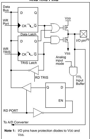
FIGURE 5-2: BLOCK DIAGRAM OF RA4/T0CKI PIN
