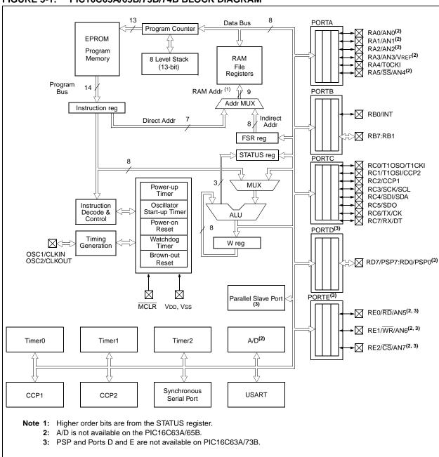
FIGURE 3-1: PIC16C63A/65B/73B/74B BLOCK DIAGRAM
