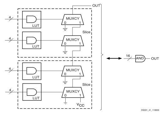
Figure 26: Wide-Input AND Gate (16 Inputs)
