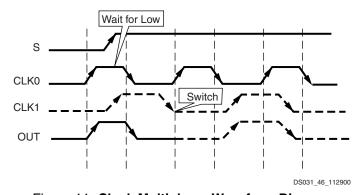
Figure 44: Clock Multiplexer Waveform Diagram
