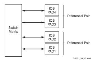
Figure 1: Virtex-II Input/Output Tile
