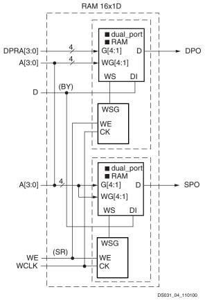
Figure 20: Dual-Port Distributed SelectRAM (RAM16x1D)
