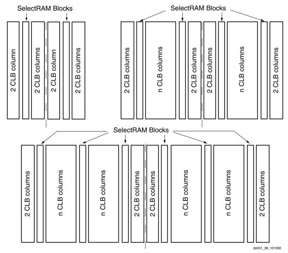
Figure 34: Block SelectRAM (2-column, 4-column, and 6-column)
