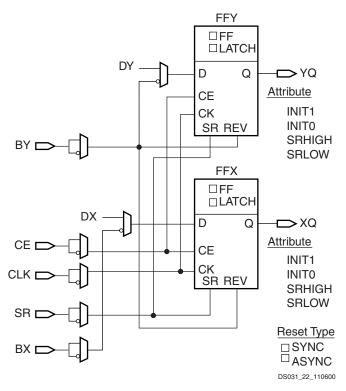
Figure 17: Register / Latch Configuration in a Slice
