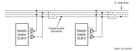
Figure 28: 3-State Buffer Connection to Horizontal Lines
