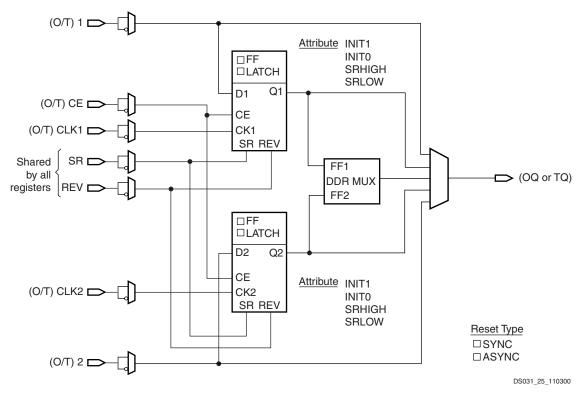
Figure 4: Register / Latch Configuration in an IOB Block
