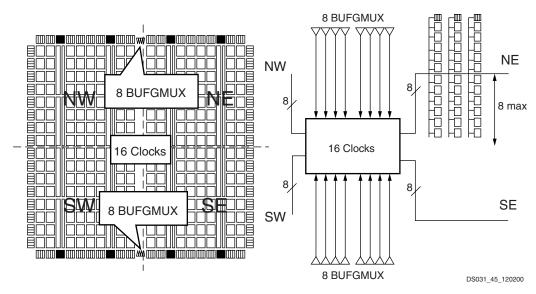
Figure 40: Virtex-II Clock Distribution
