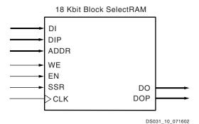
Figure 29: 18 Kbit Block SelectRAM Memory in Single-Port Mode
