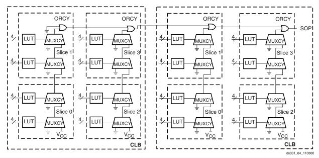
Figure 25: Horizontal Cascade Chain
