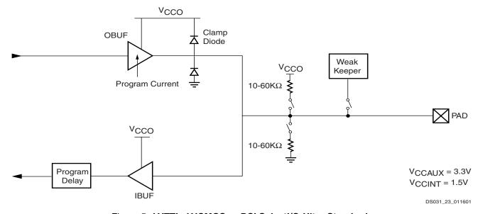
Figure 5: LVTTL, LVCMOS or PCI SelectI/O-Ultra Standards
