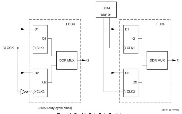
Figure 3: Double Data Rate Registers
