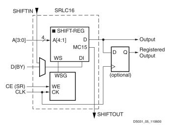
Figure 21: Shift Register Configurations
