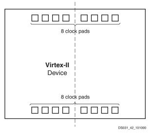
Figure 38: Virtex-II Clock Pads
