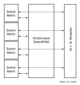
Figure 35: SelectRAM and Multiplier Blocks
