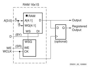
Figure 18: Distributed SelectRAM (RAM16x1S)
