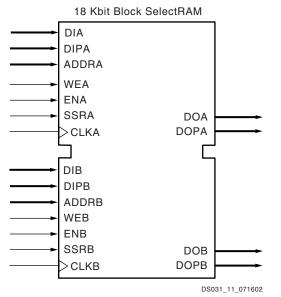
Figure 30: 18 Kbit Block SelectRAM in Dual-Port Mode
