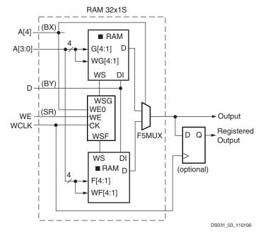
Figure 19: Single-Port Distributed SelectRAM (RAM32x1S)
