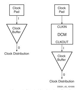
Figure 39: Virtex-II Clock Distribution Configurations
