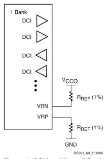
Figure 9: DCI in a Virtex-II Bank
