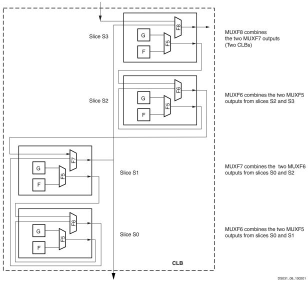
Figure 23: MUXF5 and MUXFX multiplexers
