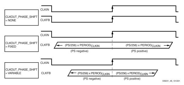
Figure 46: Fine-Phase Shifting Effects
