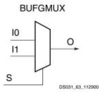
Figure 43: Virtex-II BUFGMUX Function
