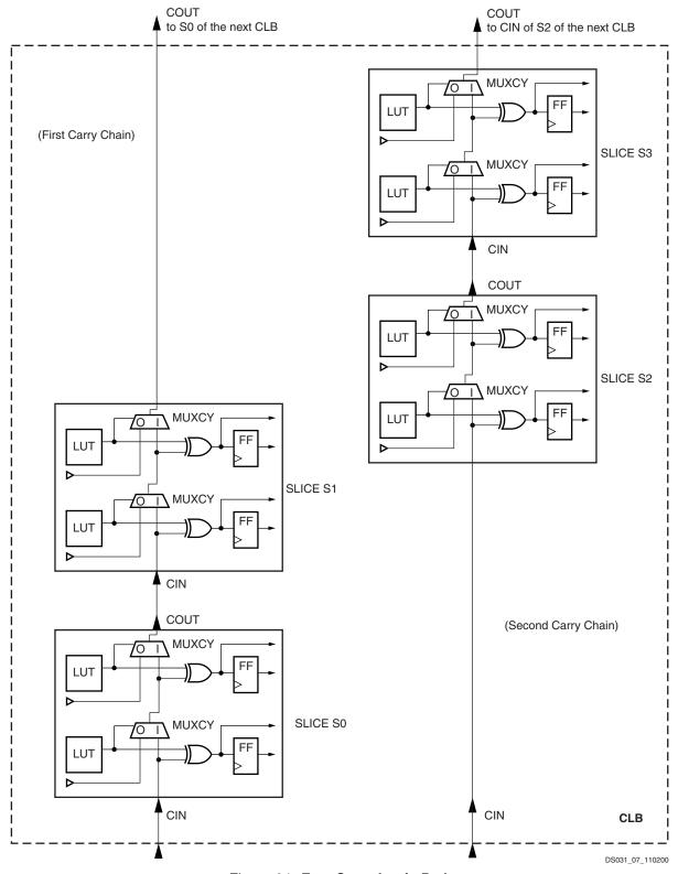
Figure 24: Fast Carry Logic Path
