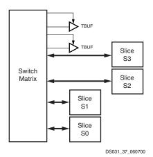
Figure 27: Virtex-II 3-State Buffers
