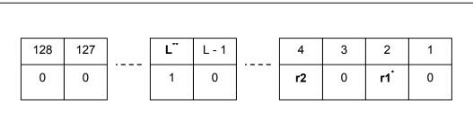
\* **ROM\_ID** bits corresponding to the **id\_bit\_number** from a previous search \* **LastDiscrepancy** bit position
