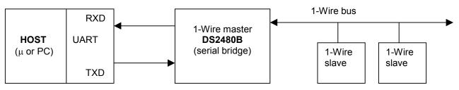
The minimum host UART that will work with this bridge must support 8-bit, non-parity, 9600 baud (bits per second) communication. Faster data rates up to 115200 baud can be negotiated but the bridge starts at 9600 baud when powering up. Electrical considerations such as RS232 are addressed in DS2480B data sheet.
